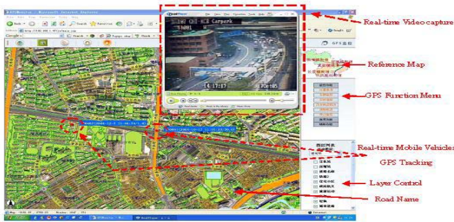
Fig. 6. The Screen Copy of Real-time Monitoring of Mobile Vehicles and Video Capture of a Road Cross
